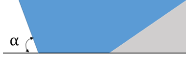
Figure 4: The supported surface. If the angle \alpha between the part surface and the horizontal axis is smaller than 45 degrees, support structure should be added. The gray area shows the added support structure.
